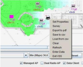
conditions as they are likely to obtain in the real world. This is the user interface for the VSS: a robot symbol that can be defined and be moved anywhere. As the control window shows a survey can be saved and recalled as well as printed for later reference.
