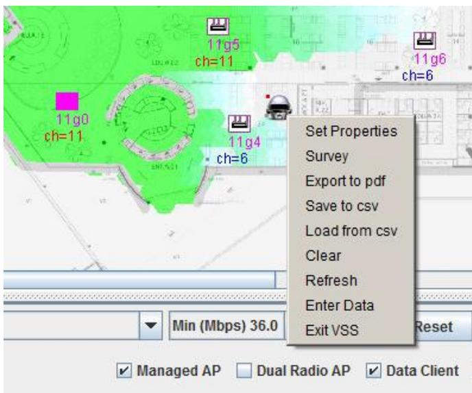
At each location, the VSS shows the local signal conditions as shown in the picture below
